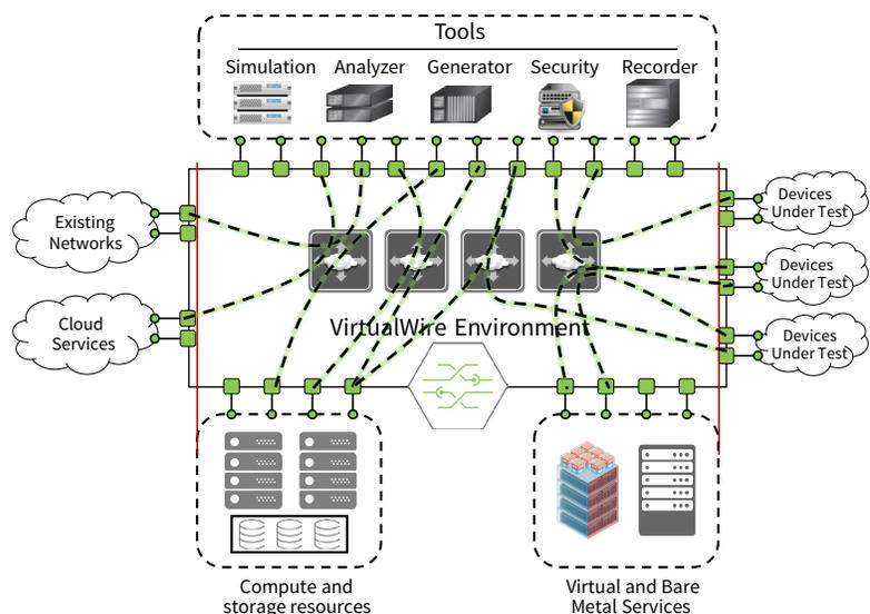
The VirtualWire solution provides physical layer 1 connectivity enabling interconnected devices see each other as being directly connected with all frames transparently passed-through the interconnected ports
