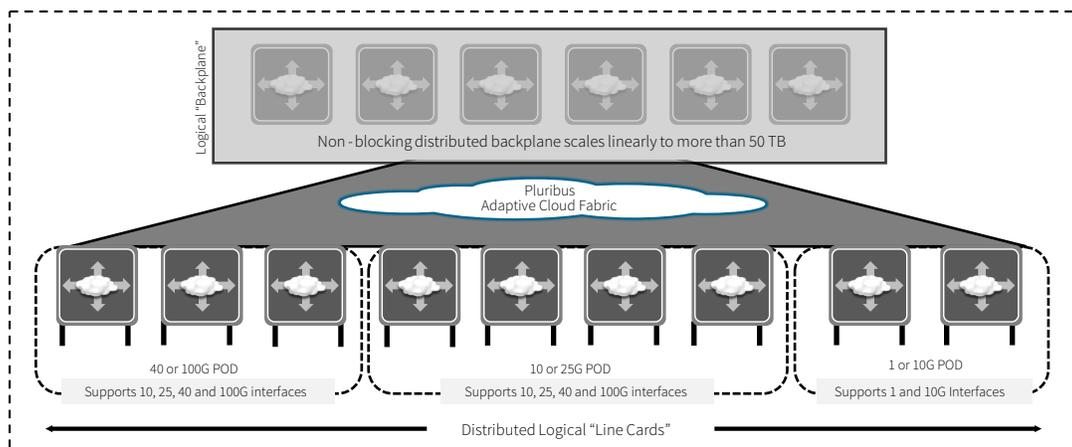
Scale-out Pluribus VirtualChassis located in a single rack, distributed across top of rack, or deployed in geographically distributed locations
