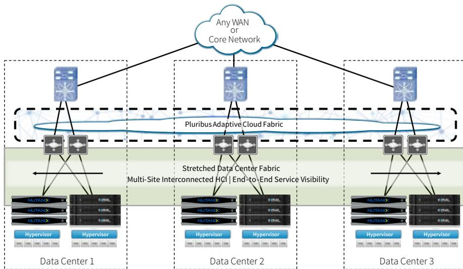
The Adaptive Cloud Fabric stretches distributed Hyper-Converged Infrastructure deployments across multiple data centers for synchronous replication and active-active HA/DR requirements
