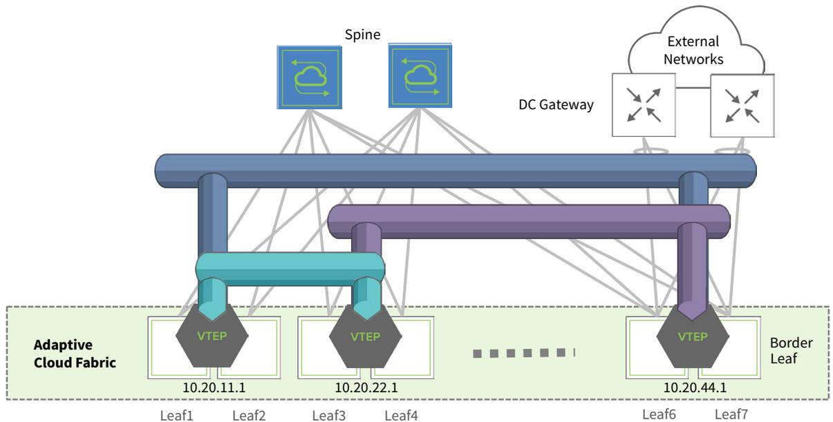
With the Adaptive Cloud Fabric control-plane, the instantiation of VTEP objects triggers the automatic creation of all the required VXLAN tunnel connections in both directions between switch clusters, resulting in a significantly lower amount of time for configuration efforts.
