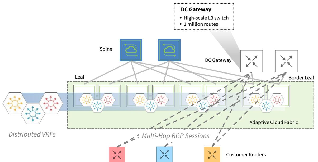
The DC Gateway function, aggregating all external and internal network routes for all tenants, must be capable of scaling to the order of one million routes, one thousand VRFs and one thousand BGP sessions.
