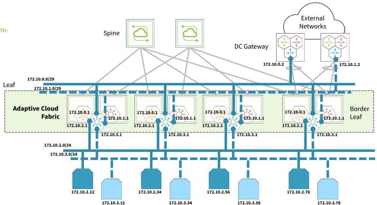
As represented in Figure 9, the overlay VRF discussed is now provisioned with two additional northbound subnets with subnet mask 29, that provide reachability in and out the VRF from/to the DC gateway:
