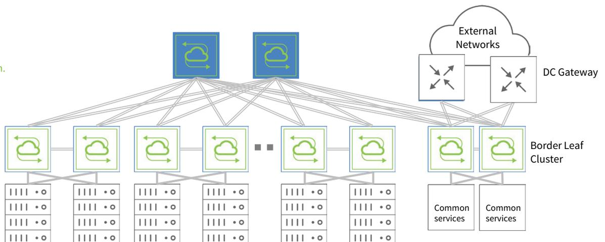
If higher capacity is desired, the topology can be expanded to 32 leaf switches by adding two additional Freedom 9532-C switches. As a result, the Clos fabric can scale up to 1536x10G access ports with 1.2:1 oversubscription ratio, as represented in Figure 2.
