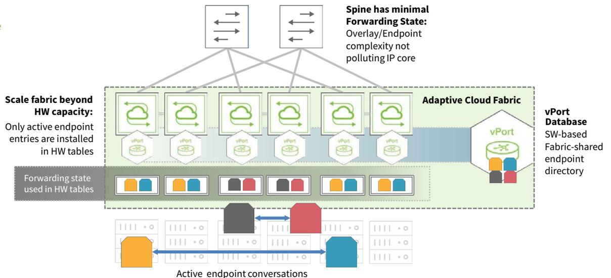
The Adaptive Cloud Fabric implements very sophisticated fabric's control plane logic that significantly reduces the dependency of hardware tables for synchronizing the endpoint database across Fabric members as it occurs with standard EVPN, and instead uses a more optimized mechanism based on the versatile vPort database.
